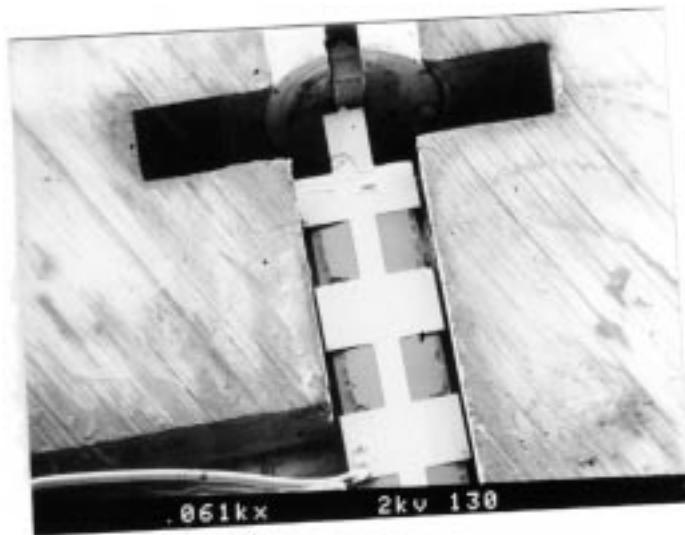
Fig. 6. Assembled and contacted tripler circuit.
